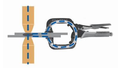
When E-Coats, primers, adhesives and other non-conductive coatings are present and squeeze-type resistance spot welding (STRSW) is required, successful welds can be made using Pro Spot Shunting Pliers. Superior engineering helps improve current flow that allows maximum resistance to be created when starting a series of spot welds.
