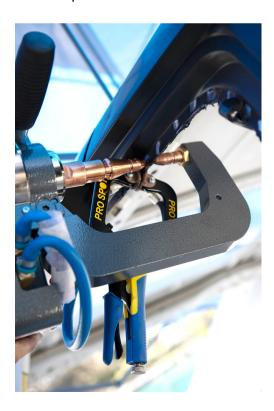
Better Connectivity Through Better Engineering - unlike other shunting pliers, Pro Spot Shunting Plier utilizes a conductive through washer to connect the first weld site to start welding. Pro Spot Shunting Plier quickly flows the current from one side to the other. copper wire and the electrodes. This prevents damage and diminished current flow over time.
