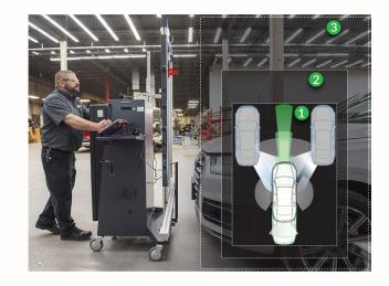
The majority of forward-facing ADAS calibrations can be completed within 16.5 feet or less.
