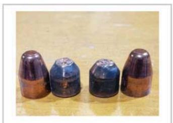
When the caps are too short the welds tend to blow out due to loss of pressure at the tips.
